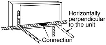
There are 4 directions allowed, namely, horizontally perpendicular to the unit, vertically down from right, horizontally out from right and horizontally out to left. Don't form the piping downward at the left of the unit.
