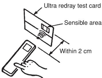
The sensible area should flash in orange when you operate the remote control unit if it is good.
