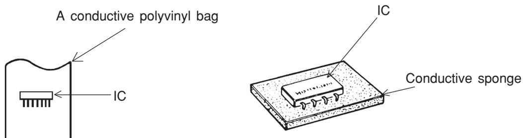
Fig. 1. Conductive Container
