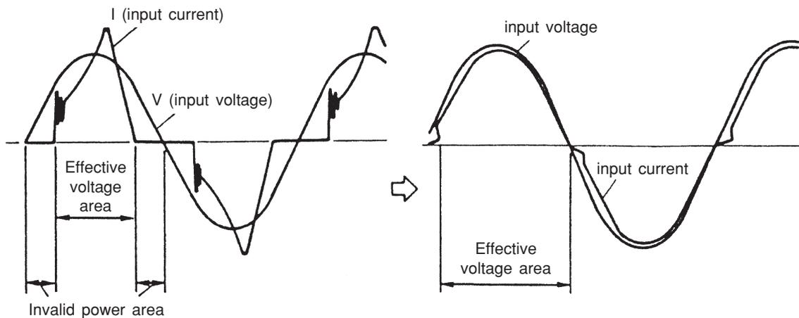
(Even if voltage is applied, current does not flow)
