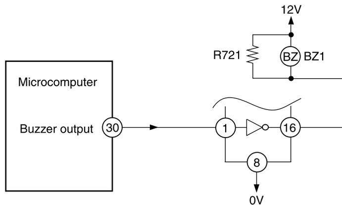
Fig. 3-1 Buzzer Circuit
