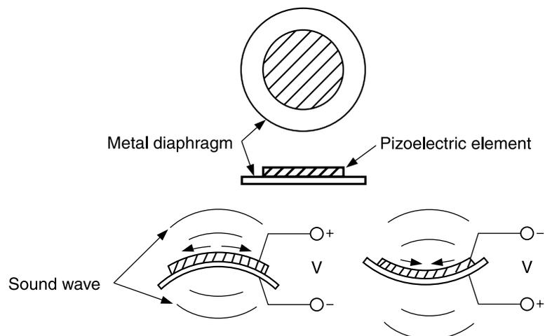
Fig. 3-2 Buzzer Operation
